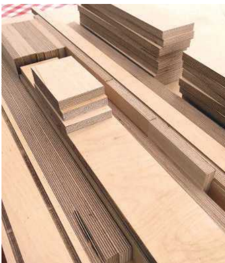
▲ Pic.7 Quality ply is a great material: strong, stable, uniform and decorative. A stack of components precisely cut is anticipation embodied. But notice scorch marks: some seemed inevitable and had to be accepted. Furniture made of ply is only ever that and on the grand scale will not be 'fine'
